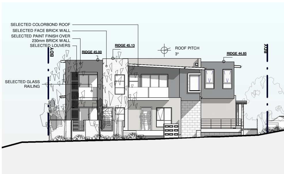
1 FRONT ELEVATION- NORTH DA300 1 : 200
